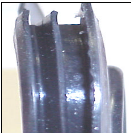
Brake Master Cylinder Rubber Cross Section ~0.50 Inch Across
